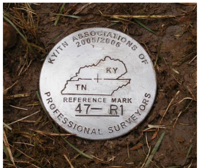
Typical reference monument set to preserve the location of stone markers when found.
